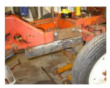
I used a pair of ½ drive socket U-joints to replace the massive U-joints used in steering shaft of the original tractor. This was done to reduce the length of the joints. The control valve shaft has to be cut off as short as possible to allow room for the hoses to come out the bottom of the valve.
