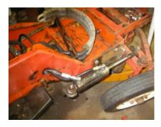
Here is a picture of the return hoses from the control valve and the spool valve T'd together and routed to the oil cooler. The T fitting is from the Sunstar.
