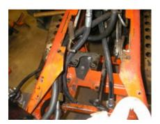
Next the input shaft to the control valve has to be cut off short to allow room. I cut the shaft and outer housing off at the length I wanted the shaft to be and then cut the outer housing. There is a plastic support bushing and a rubber seal that are re-installed from the cut off portion of the shaft.
