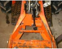
The Sunstar steering cylinder can be installed with or without the front plow/snow blower bracket, which is shown in the picture below.
