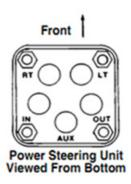
The IN port is connected to the main hydro power beyond output port.
