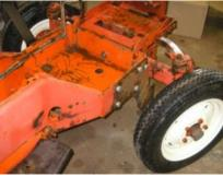
A new mounting bracket for the steering cylinder was fabricated using 3x3 angle iron. This bracket bolts over the plow bracket using the lower two bolts that attach the plow bracket. This configuration was chosen to allow the cylinder sufficient clearance when the axle is pivoted to it's extreme positions.
